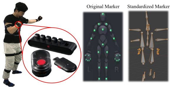
Figure 1: The motion capture equipment used in our data collection process, featuring the optical tracking system and marker set that enables precise 3D tracking of body movements. The markers are strategically placed at anatomical landmarks to enable precise tracking of all major body segments during movement.
